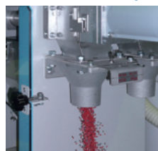
残材抜き Extraction of Remaining Materials
