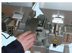
計量チェック扉開 Measuring Test Door Opens
