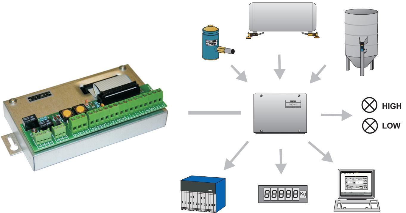
The S-E-G system W3 transmitter is used for analog load cell to digital conversion, level control and weight/signal monitoring via RS485 serial communication, or 4-20 mA analog output current signal. The load is sensed by Strain gauge loadcells selected for the desired load range. The transmitter is also available in stainless field enclosure for use in harsh industrial environments requiring heavy duty equipment with high reliability and IP65 protection.
