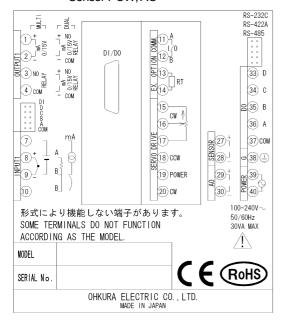
2) EC5900R: DI/DO terminal adapter, ARCNET, Servo drive, Sensor POW, AO
