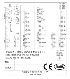
3) EC5900R: DI/DO connector, RS-485, Sensor POW, AO EC5950R: DI/DO connector, RS-485, Sensor POW, AO
