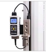
Indicator / load cell adapter Accommodates any Mark-10 indicator and Series R01 or R03 force sensors. Includes mounting hardware.
