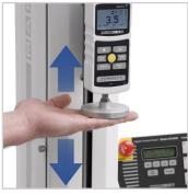
**FollowMe**<sup>™</sup> Using your hand as your guide, push and pull on the load cell or force gauge to move the crosshead. Responsive enough for quick positioning as well as fine adjustments.
