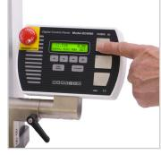
Simple controller interface Rugged aluminum keys are designed for industrial environments, with dedicated Zero Travel and FollowMe™ keys. Removable for remote use.
