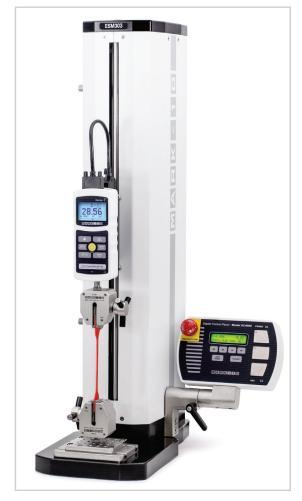
ESM303 is shown above configured for a tensile test, with a Series 7 force gauge and G1061-2 wedge grips.
