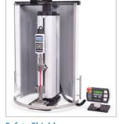
Safety Shield Provides pinch and sample debris protection for the operator. An electrical interlock prevents test stand operation while the door is open.
