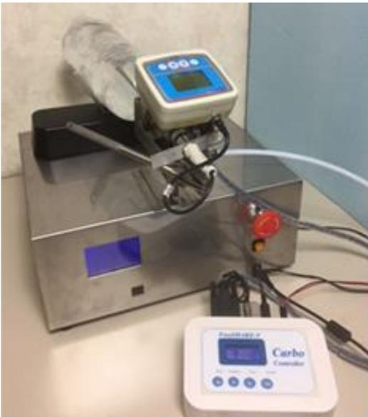
FreeSHAKE-V CARBO is a mini carbonator that assists your new product development of carbonated drinks. Accurate carbonation to the target gas volume will be available in a short time by a simple operation. Any size of package is applicable, from a small bottle less than 100ml to a big container over 3000ml.
