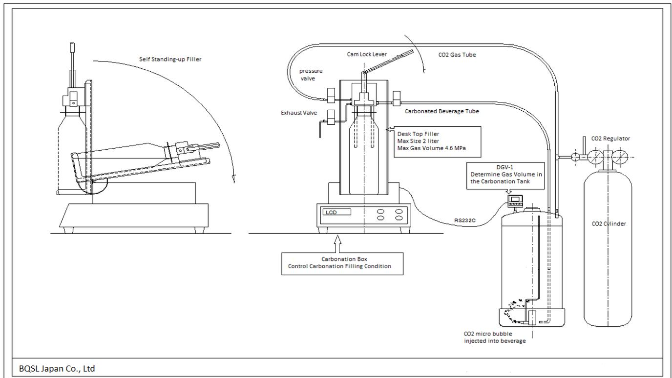
High performance micro bubble carbonator tank is a size of 20 liter. It has a pressure-resist small micro bubble generator at a bottom of the tank. CO<sub>2</sub> gas is injected in the beverage to be micro bubbles, and the gas is dissolved in very effectively. High performance micro bubble carbonator tank is equipped with DGV-1 which measures gas volume in real time. When the gas volume reaches the setting value, it alarms you with a buzzer.
