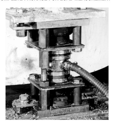
The Weigh Module M is a load sensing component in S.E.G. scale systems.
